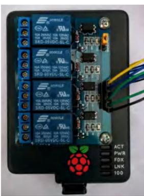
Control relays connected to you RaspberryPi using Android app. Setup multiple RaspberryPi devices around your house. Single device can operate up to 8 relays and all of them are self-discoverable...
