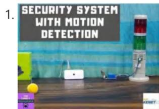
1. The system is designed to detect intrusion (unauthorized entry) into a building or other area. Step 1: Things Used in This Project Hardware components KEMET Electronics Corporation Proximity Sensor- Pyroelectric...
