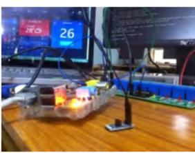
Components Required Raspberry Pi Sensors - Temperature sensor (DS18B20) 8 Channel Relay (12V/ 7A/ 240 V AC) Bulb (60W)
