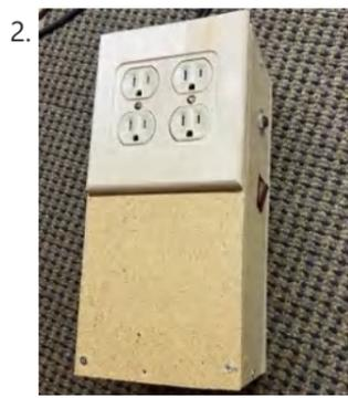
2. I made a power strip that has 4 independently switchable outlets from a raspberry pi and other materials that I mostly had sitting around. The raspberry pi is running Homebridge...
